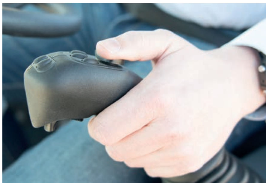
For frequent steering, the Adjustable Joystick Steering option allows to control the machine with less effort
