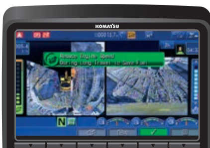
Eco-gauge, Eco guidance and fuel consumption gauge
