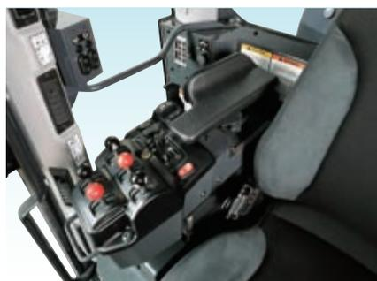
*The arm console height can be electrically adjusted*
