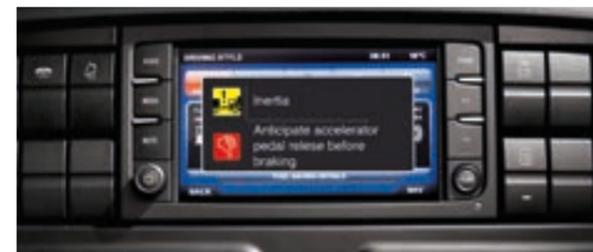
**Fuel-saving suggestions** appear on screen while the vehicle is running (they taking into account gears, braking, engine braking, acceleration and inertia).
