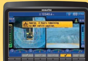
AdBlue® level and refill guidance
