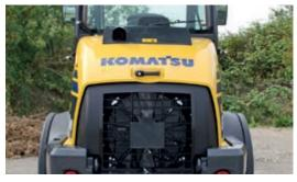
The Komatsu EU Stage V engine is productive, dependable and efficient and offers increased engine power. It requires no Adblue® to meet emission standards.
