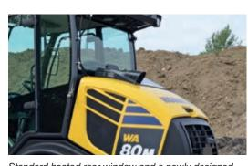
Standard heated rear window and a newly designed, low-profile exhaust pipe ensure improved rear visibility (to ISO 5006).
