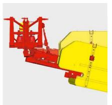
The mower is lowered so that the outer end of the cutter bar contacts the ground first. At the headland, the inside end is lifted first. That is how your sward is perfectly protected.
